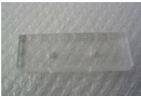
Figure 21. Plexiglas substrate used in the fabrication of microfluidic devices with two holes.
