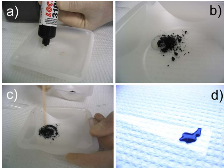
Figure 30. a) Dispense Loctite into a plastic dish. b) Add magnetic particles. c) Mix by hand or use a homogenizer. d) Transfer the mixture to a substrate and expose to UV light.
