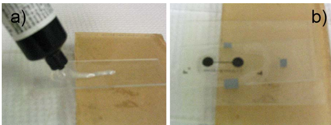
Figure 26. a) The 3108 is dispensed onto the glass substrate and b) covered with a mask coated with Sylgard 184 elastomer base. The gray squares are silicon wafer pieces 500 \mu\text{m} thick that are used as spacers to give a defined film thickness.
