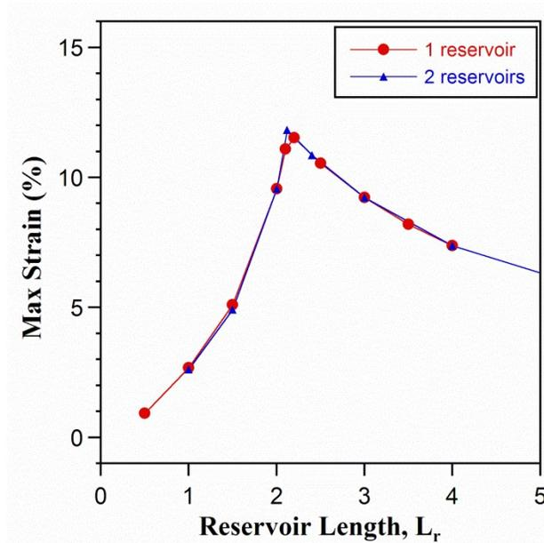
Figure 3. Maximum strain as a function of total reservoir length for one versus two reservoirs.
