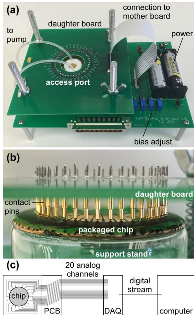
**Figure 4.** a) Overview of the PCB boards used to contact the chip. b) The daughter board had spring-loaded pins to contact the chip package and a cable to the mother board. The mother board included batteries for power, pots for adjusting the on-chip transistor biases, and a cable connector. c) The PCB was connected to a data acquisition system that converted the analog data to digital signals, which were transmitted to a laptop for recording and later analysis.
